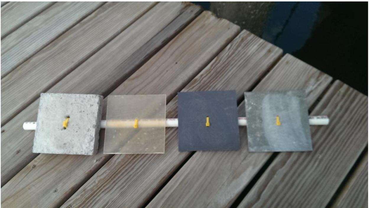
Figure 1. General set up of a set of four 14x14cm fouling plates attached to a PVC pipe with zip ties. Order of plates from left to right: Concrete, Fiberglass, PVC, and Slate.
