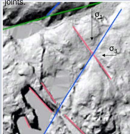
**Figure 2.** represents  $\sigma_1$  (maximum principal stress) and  $\sigma_3$  (minimum principal stress).
